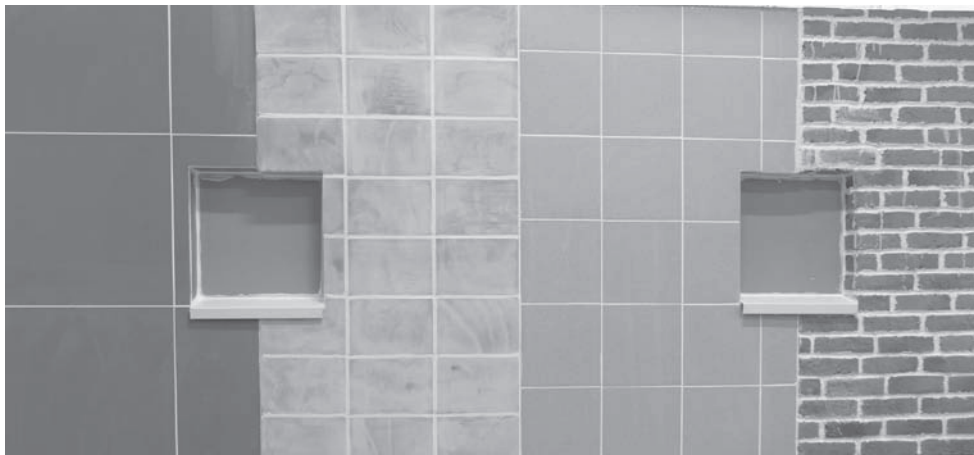
Fig.1 The specimen used in the study. The specimen was prepared from (starting from the left): ceramic tiles, 0.6x0.6 m size; natural sandstone cladding, 0.3x0.2 m size; ceramic tiles, 0.3x0.3 m; concrete tiles 0.2x0.1 m size. All the claddings were glued to the wall with C2TE class tile adhesives according to EN 12004 standard.
